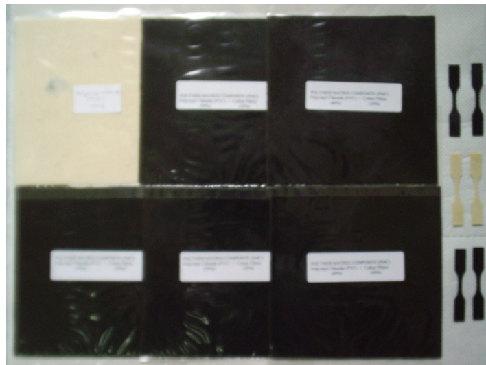
Figure 2. Set of pressed PVC specimens.
