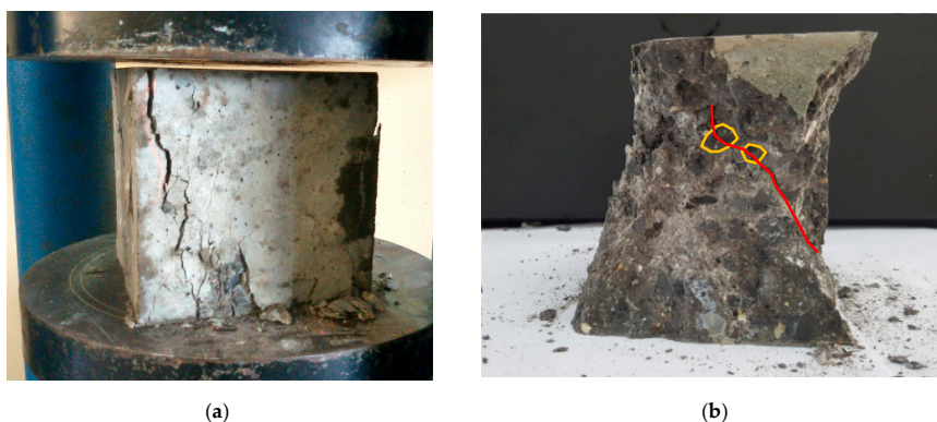
Figure 5. Typical crack under compression of 100 mm cube specimen of the steel-slag concrete. (a) Failure crack. (b) Cracking feature.
