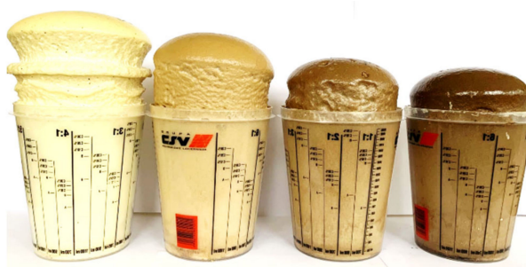
Figure 5. PUR foams obtained in the study: (a) WS-0%, (b) WS-10%, (c) WS-20%, and (d) WS-30%.
