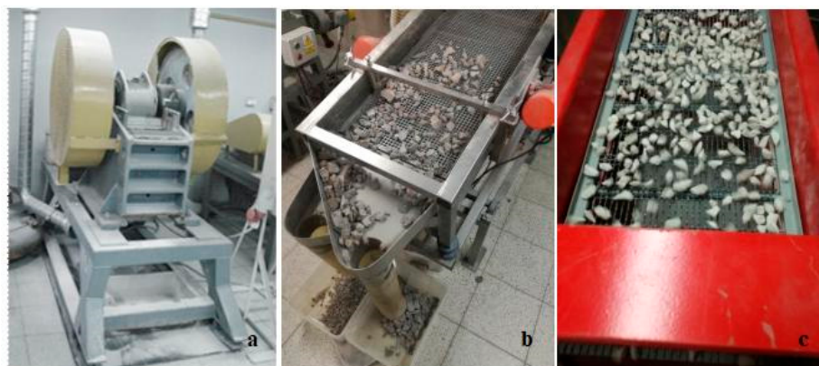
Figure 2. Jaw crusher (a), double deck vibrating screen (b), and vibrating screen with slotted sieves (c).
