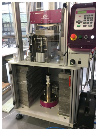
Figure 7. The impact drop tower for dynamic loading experiments.
