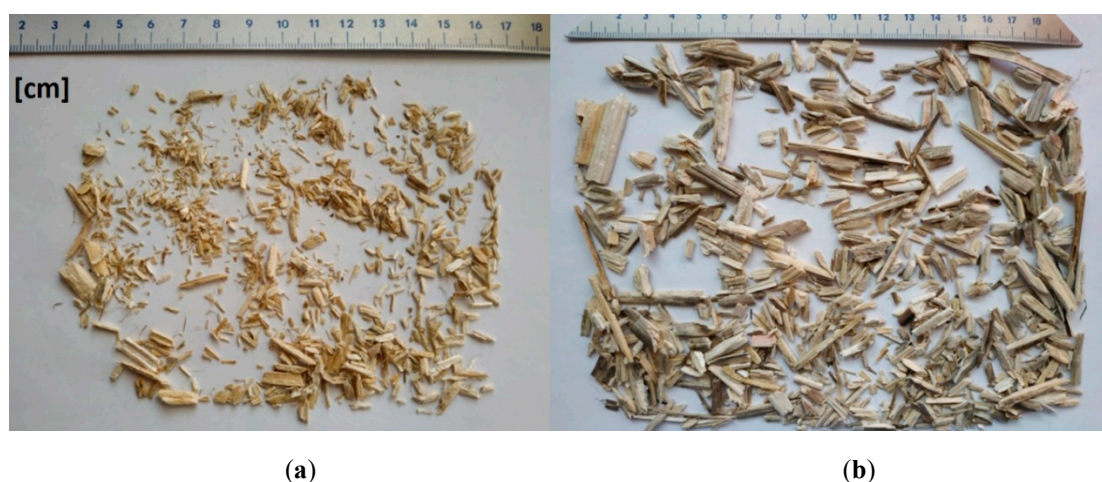
Figure 1. Hemp shives used in the investigation: fine shives (a) and thick shives (b).
