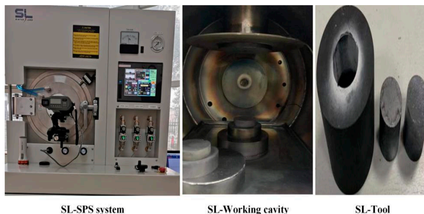
Figure 3. SL-spark plasma sintering (SPS) equipment (Sinter Land Iinc, Niigata Prefecture, Japan).
