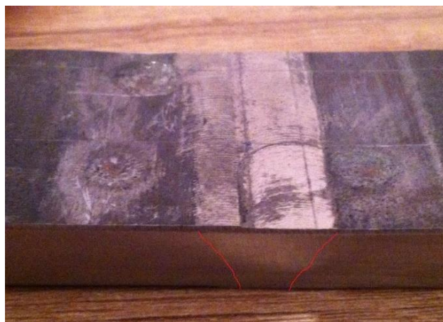
Figure 11. Damage in the base metal of the 1.29 kJ/mm weldment: plastic flow (shots 13, 14 and 15).
