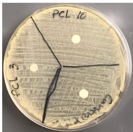
Figure 15. Inhibition zone experiment on a control, PCL-3, and PCL-10 disc in a TSA agar plate.
