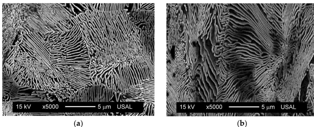
**Figure 3.** Microstructure in the longitudinal sections of the analysed pearlitic steel wires at different degrees of drawing: (a) hot rolled wire E0 (not cold drawn) and (b) moderately cold drawn wire E3.
