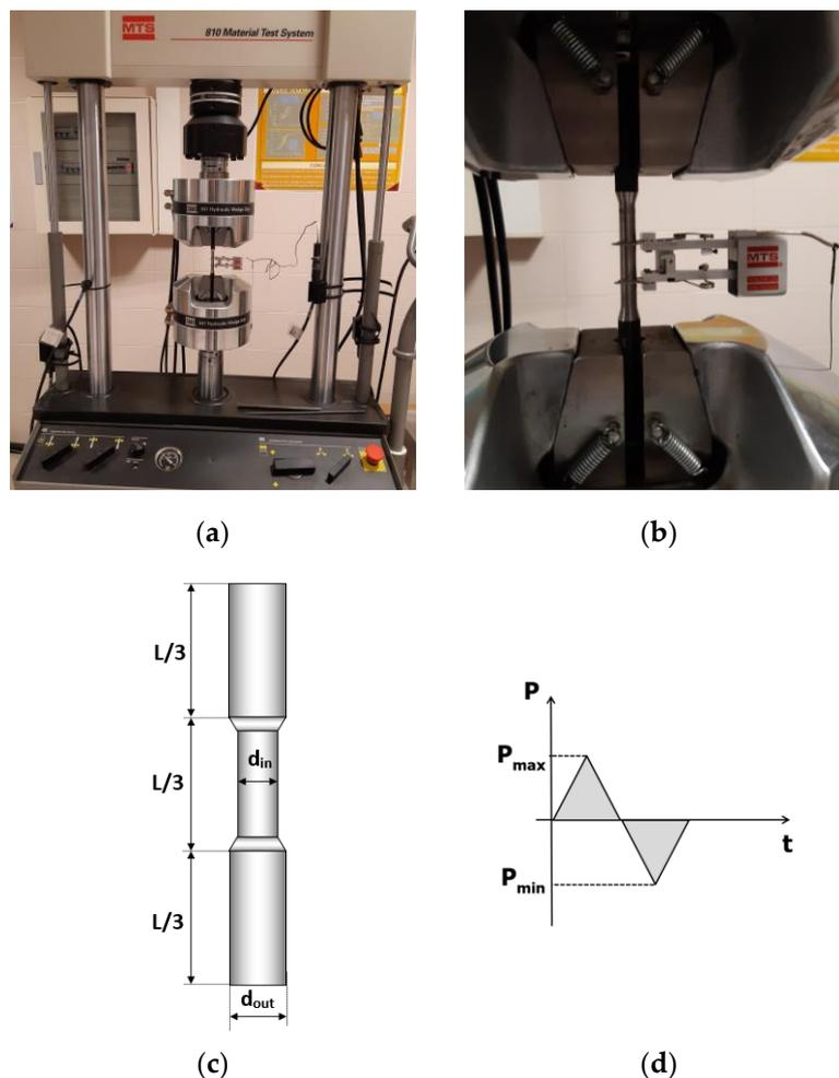
**Figure 5.** Experimental set up: (a) test machine used for Bauschinger test, (b) detail of the test specimen with the extensometer, (c) scheme of the specimen geometry and (d) scheme of the applied load route.
