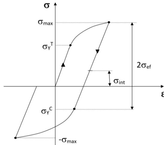
**Figure 2.** Definition of the effective and internal stresses.
