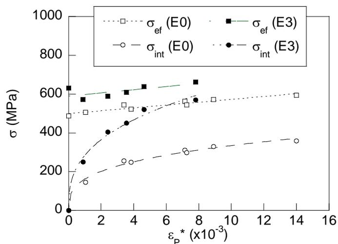
**Figure 9.** Evolution of the internal and effective stresses with plastic pre-strain for the steels E0 (open symbols) and E3 (full symbols).
