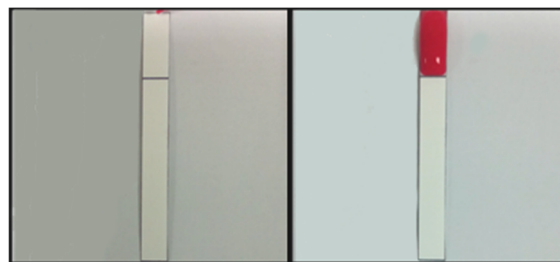
Figure 3. Barrier penetration test. (Left): Surfactant solution in 0.5 \mu L was added at the front of the barrier and dried for 1 h; (Right): phosphate-buffered saline (PBS) (100 \mu L) was added for penetration.
