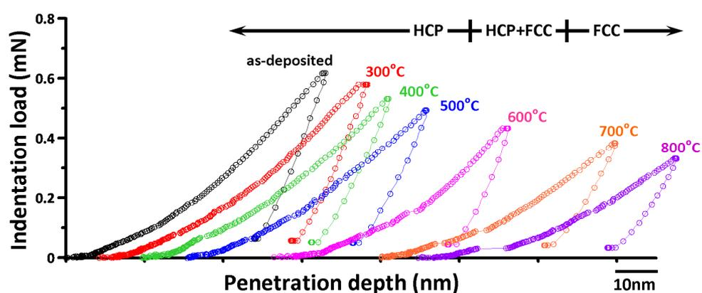
**Figure 2.** The continuous stiffness measurement (CSM) load-displacement curves of the as-deposited Co film and those being annealed at various temperatures, ranging from 300 °C to 800 °C.
