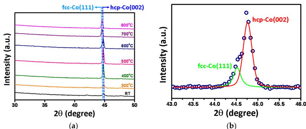
**Figure 1.** (a) X-ray diffraction (XRD) patterns of the as-deposited Co thin film, and those being annealed at temperatures of 300 °C–800 °C. (b) The fitting data of XRD result for 600 °C-annealed Co thin film, indicating that the coexistence of hcp-Co (002) and fcc-Co (111) peaks, locating at  $2\theta = 44.7^\circ$  and  $2\theta = 44.5^\circ$ , respectively.
