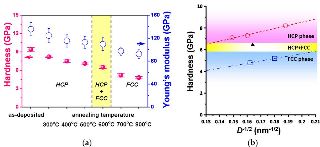
**Figure 3.** (a) Hardness and Young’s modulus of Co films as a function of annealing temperature of the as-deposited and annealed Co thin films. (b) The hardness as a function of grain size, showing similar behaviors for both the hcp- and fcc-structure Co thin films. The dash lines are the fits to the Hall–Petch equation:  $H(D) = H_0 + kD^{-1/2}$ , with  $H(D) = 28.9D^{-1/2} + 2.7$  and  $H(D) = 22.2D^{-1/2} + 1.2$  for hcp- and fcc-structured Co thin films, respectively.
