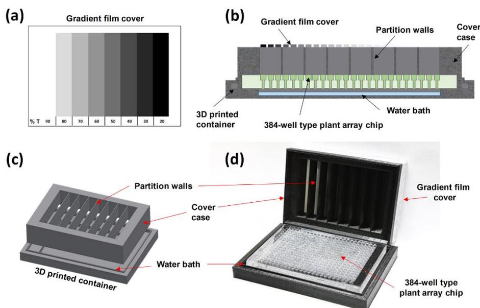
**Figure 2.** A light gradient module and the integration of a plant array chip. (a) Schematic of a laser-printed light gradient film with eight different light transmittances. % T indicates the transmittance expressed as a fraction of 100. (b) Assembly of a 384-well type plant array chip in a light gradient module. (c) Schematic of a 3D printed light gradient module case. (d) Photograph of a light gradient module and a 384-well type plant array chip.
