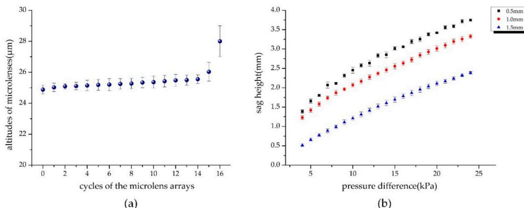
**Figure 5.** Result of morphology measurement experiment: (a) altitudes of pressed polymeric MLAs with different diameters from 0th to 16th cycles; (b) deformation of PDMS membranes with different thickness under pressure from 4–24 Kpa.
