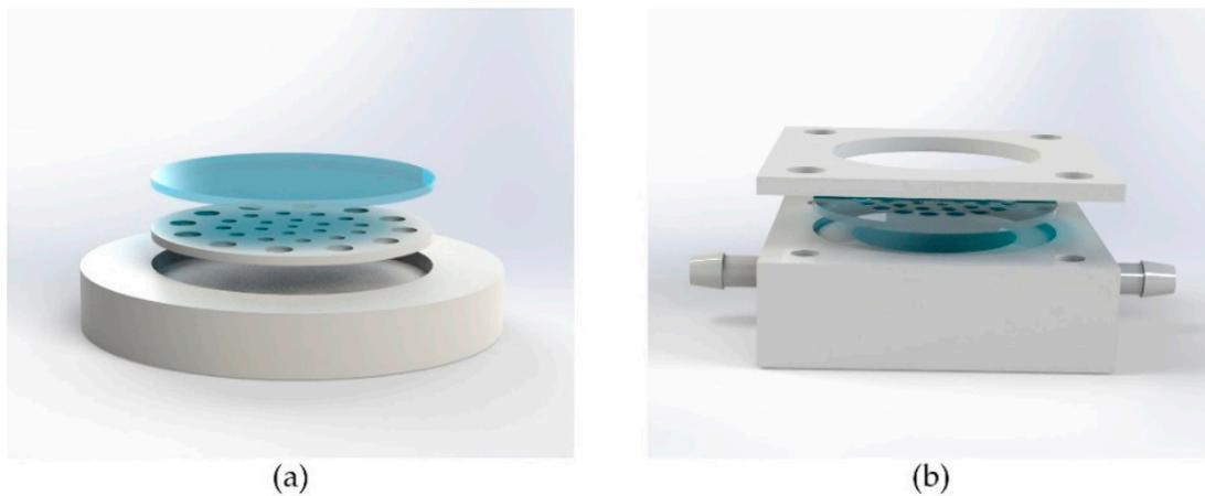
**Figure 3.** Three-dimensional diagram of the home-built metal mold structure: (a) grooved tray for relieving excess pressure in the hot embossing process; (b) sealed cavity for package of the PDMS intermediate die with MLA structure.
