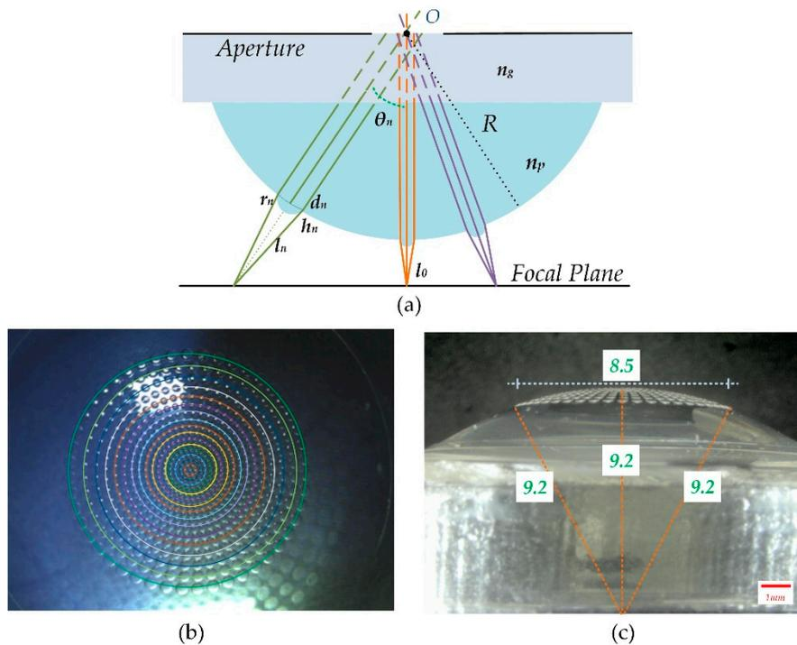
**Figure 1.** (a) Design of microlenses with multiple focal lengths on a curved surface; (b) image of curved compound eyes captured by optical stereoscopic microscope; (c) lateral view of curved compound eyes captured by digital microscope with large depth of field.
