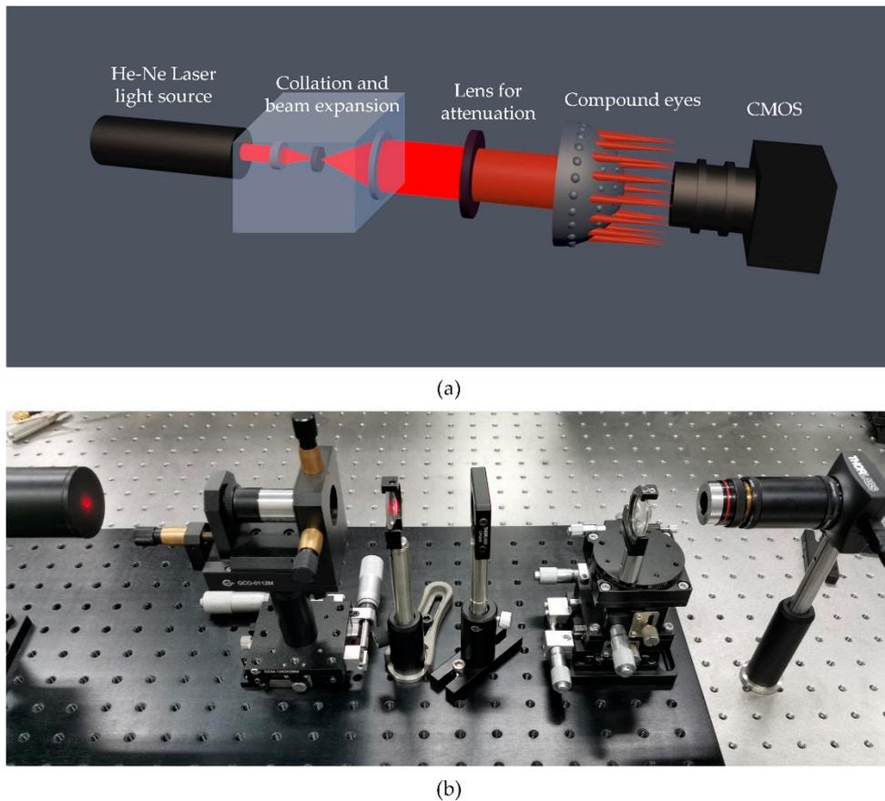
**Figure 7.** Experimental installation for optical performance: (a) schematic diagram of the setup; (b) actual platform comprised of He-Ne laser source, microscopic objective lens, pin hole, convex lens, MLAs, optical density filters, microscopic objective lens, and photodetector.
