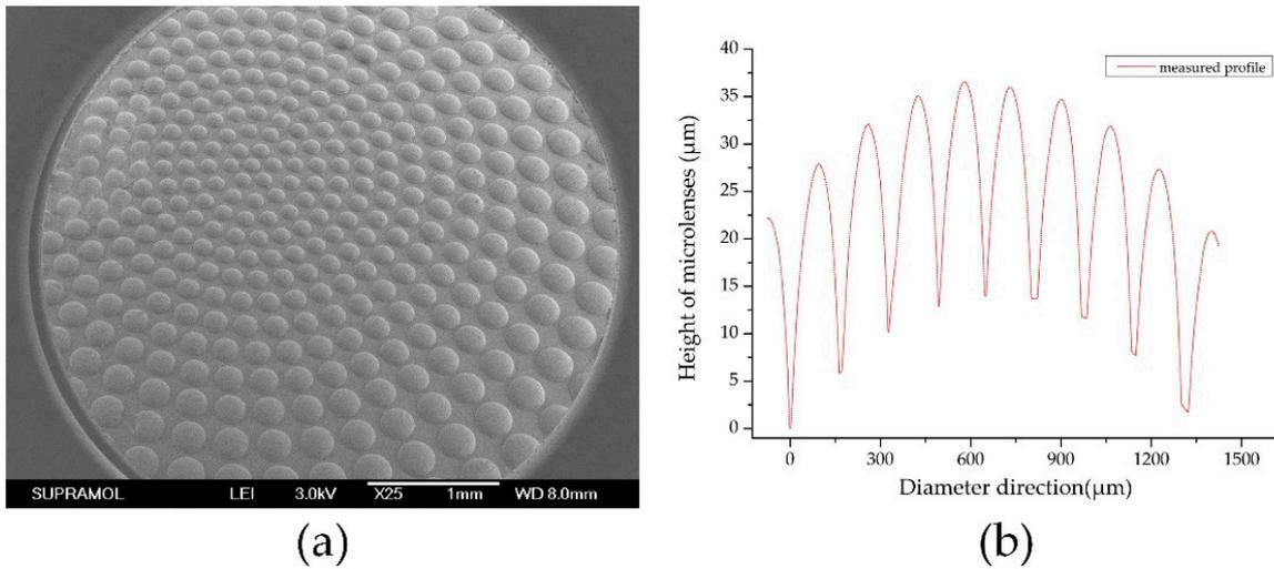
**Figure 6.** Three-dimensional (3D) profile of the compound eye: (a) SEM image of the multifocal compound eye at side view; (b) the measured profile of microlenses in center of the multifocal compound eye.
