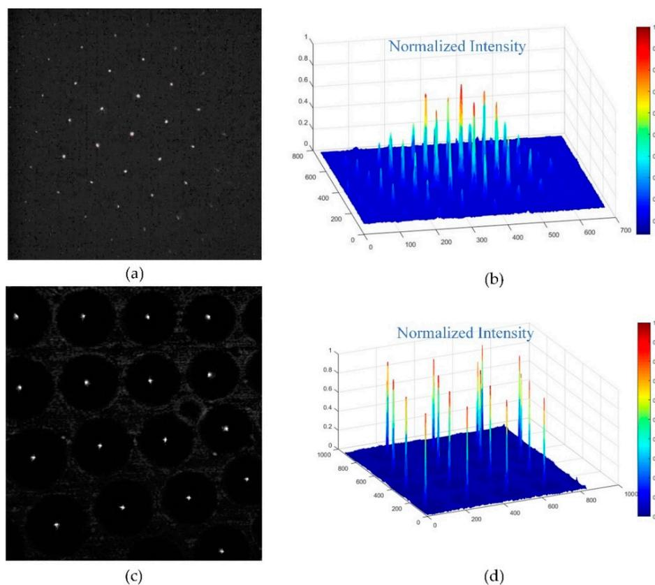
**Figure 8.** Focal spots of compound eyes with single and multiple focal lengths: (a) focal spots of single focal length microlenses on dome area; (b) normalized intensity distribution of single focal length microlenses; (c) focal spots of multiple focal length microlenses on the middle area; (d) normalized intensity distribution of multiple focal length microlenses.
