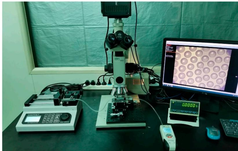
**Figure 4.** Experimental setup used to measure altitudes of MLAs with different diameters and sag height of PMDS deformation under different pressure in real time.
