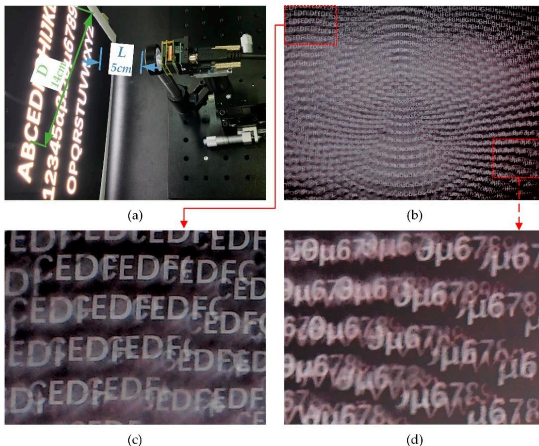
**Figure 10.** Experiment of field of view (FOV) testing: (a) experimental setup of the testing system; (b) numbers and letters captured by multifocal compound eyes; (c) close look at the upper-left portion of the image; (d) close look at the lower-right portion of the image.
