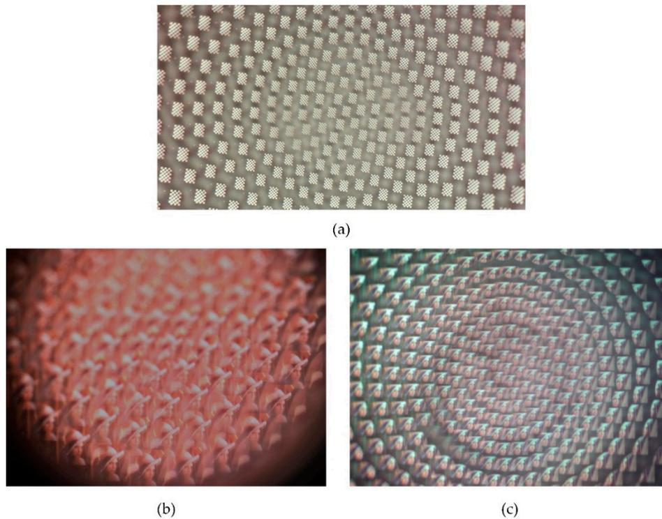
**Figure 9.** Images captured by the compound eyes: (a) calibration plate captured by the multi-focal compound eyes; (b) image of Lenna in contrast to the single focal compound eyes; (c) image of Lenna captured by the multifocal compound eyes.
