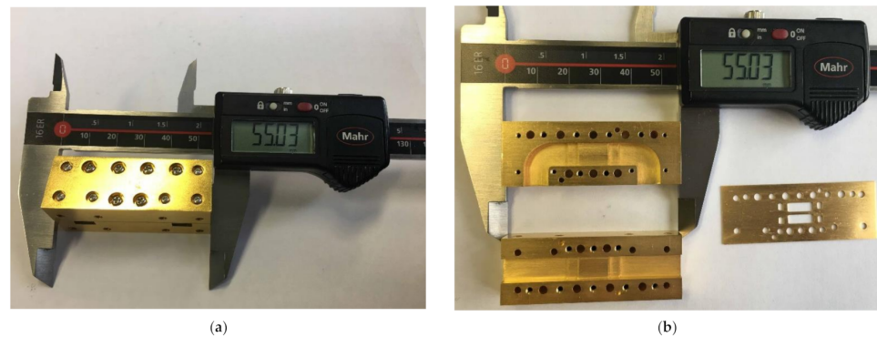
Figure 6. Photograph of sample coupler (a) assembled and (b) disassembled (the dimensions of sample coupler are 55.03 \times 20.02 \times 25.02 \text{ mm}^3 ).
