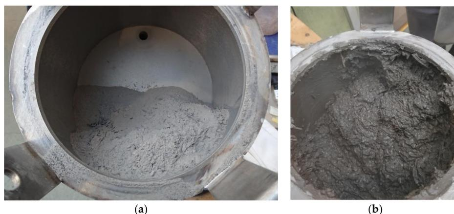
**Figure 7.** Working chamber during grinding experiments: (a) dry grinding; (b) wet grinding.
