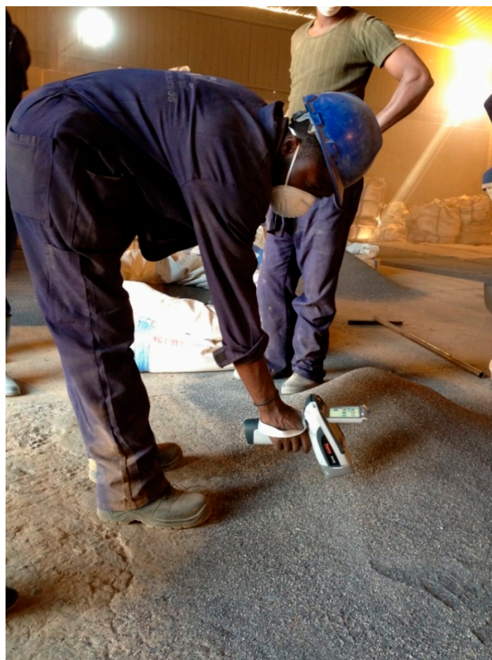
Figure 3. Analysis of coltan ore samples by HHXRF showing a real time qualitative test by the user.
