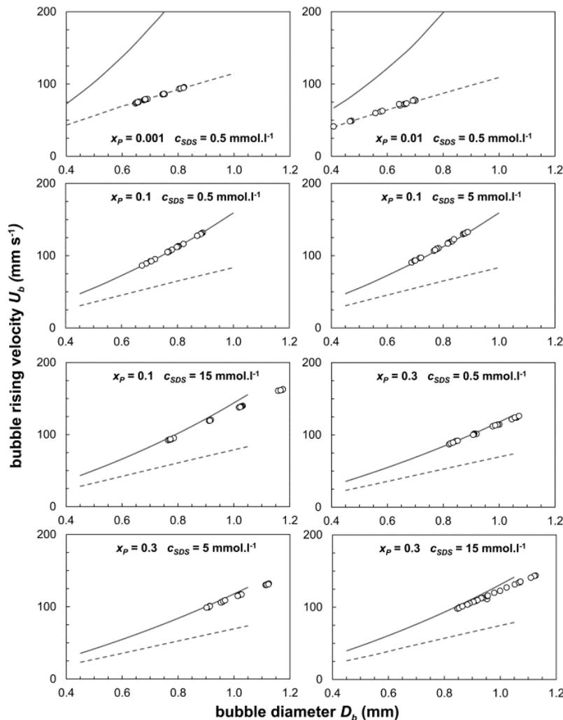
**Figure 2.** The bubble terminal velocity as a function of bubble diameter in water–propanol–SDS mixtures. The full line represents the calculated velocity for mobile bubble surface. The dashed line represents the calculated velocity for immobile bubble surface.
