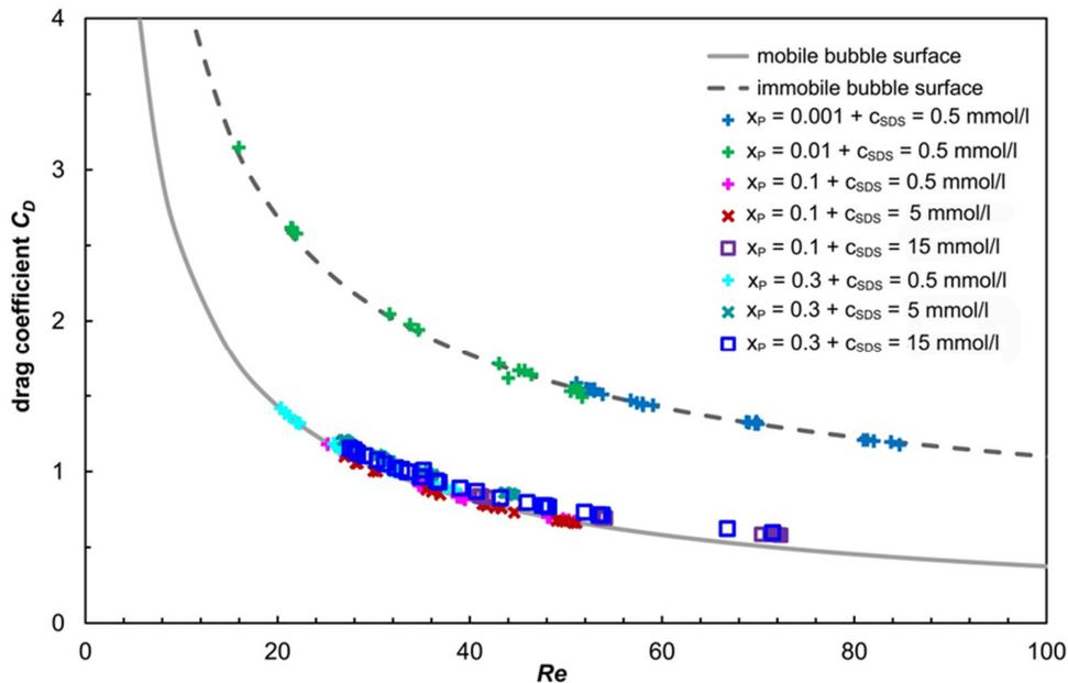
**Figure 3.** Dependence of the drag coefficient on the bubble Reynolds' number. Dashed line— $C_D$  predicted by Equation (6) (immobile bubble surface). Solid line— $C_D$  predicted by Equation (3) (fully mobile bubble surface).
