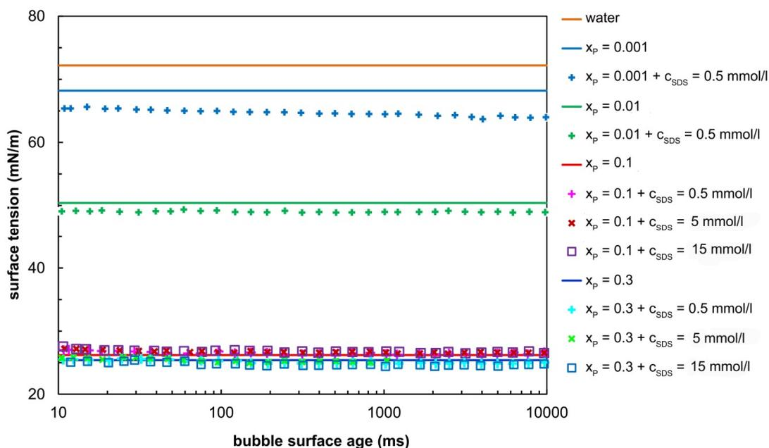
**Figure 1.** Dynamic surface tension plotted as a function of bubble surface age. The full lines represent the surface tension of water and propanol–water solutions; the symbols represent the data for the water–propanol–SDS mixture. Note: The values of surface tension for concentrated solutions ( $x_P = 0.1$  and  $x_P = 0.3$ ) overlap.
