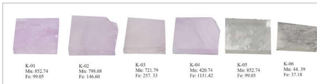
**Figure 3.** Six kunzite samples which were cut into wafers with dimensions 2 cm × 2 cm × 0.5 cm, (length, width, and thickness, respectively). These samples were used for X-ray absorption near-edge structure (XANES) and UV–VIS spectra. These samples were selected according to the Mn and Fe concentration and each sample's value is written below the sample in ppm (average).
