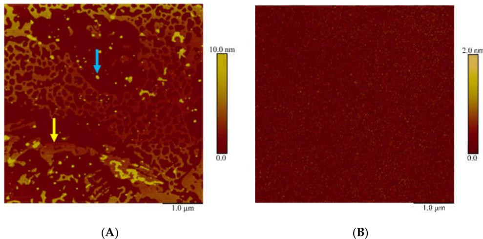
**Figure 3.** Typical AFM images obtained after incubation of DSP-activated (A) and non-activated (B) APTES-modified mica in  $10^{-9}$  M HRP solution. Yellow arrow indicates the fragment of a layer-like structure, and blue arrow indicates aggregate structures, which have been attributed to layers of immobilized HRP molecules, since no such objects were observed in control experiments.
