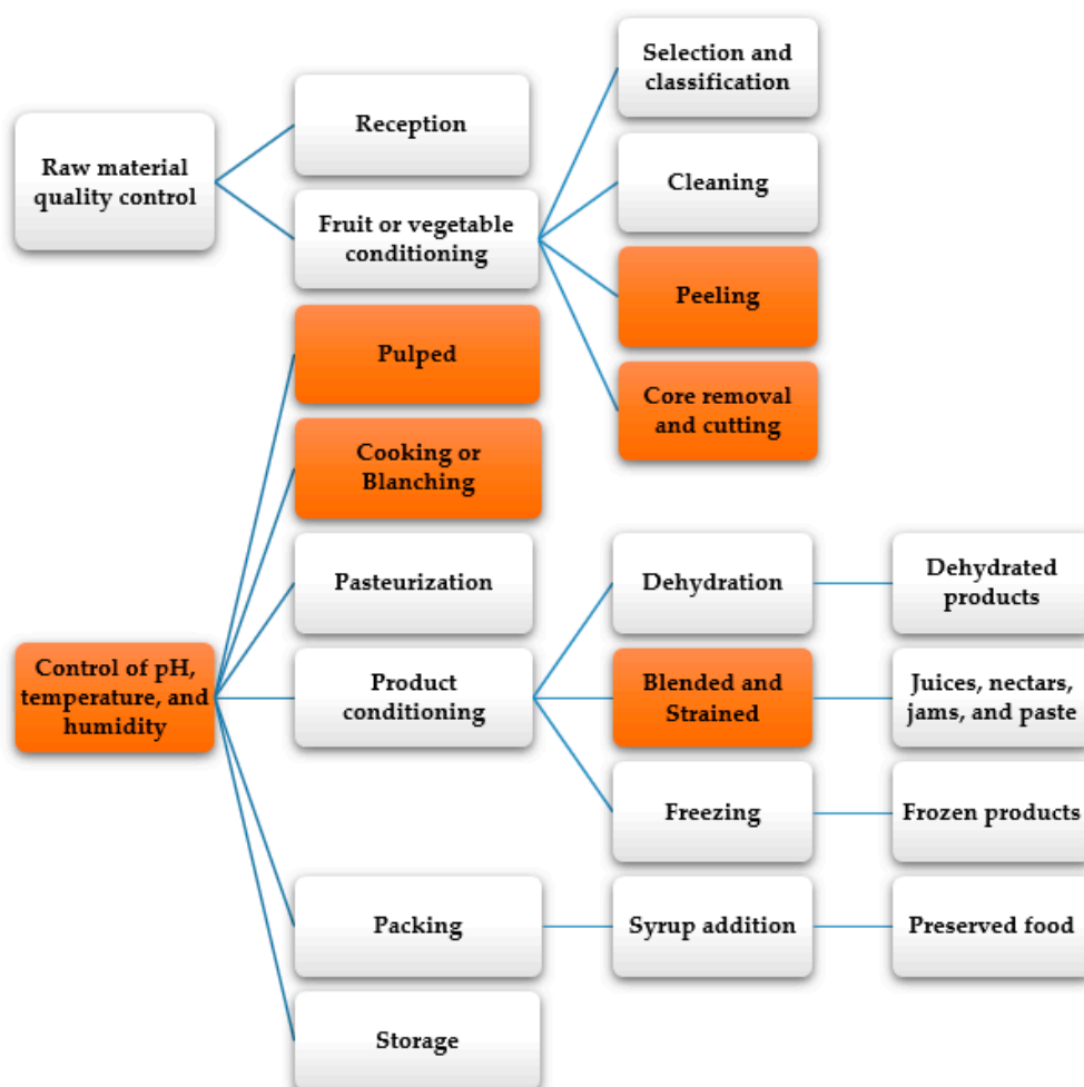
Figure 5. General diagram of fruit and vegetable industrial processing [89,90].
