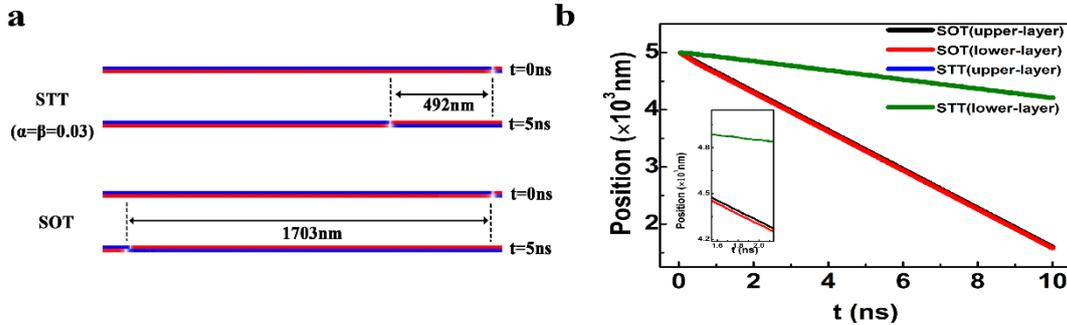
**Figure S2.** (a) The snapshots for the paired DWs driven by STT and SOT under the same current and other magnetic parameters, and (b) the temporal central positions of the upper and lower layers driven by STT and SOT ( $J_{\text{ex}} = -2.5 \times 10^{-4} \text{ J/m}^2$ ,  $D = 0.75 \text{ mJ/m}^2$ ,  $K_{\text{up}} = 6 \times 10^5 \text{ J/m}^3$ ,  $K_{\text{low}} = 2.5 \times 10^5 \text{ J/m}^3$ ).
