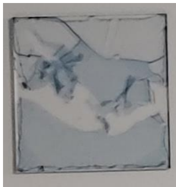
Figure S3. A photograph of the PEG vapor treated film after storage in humid chamber for 5 min.
