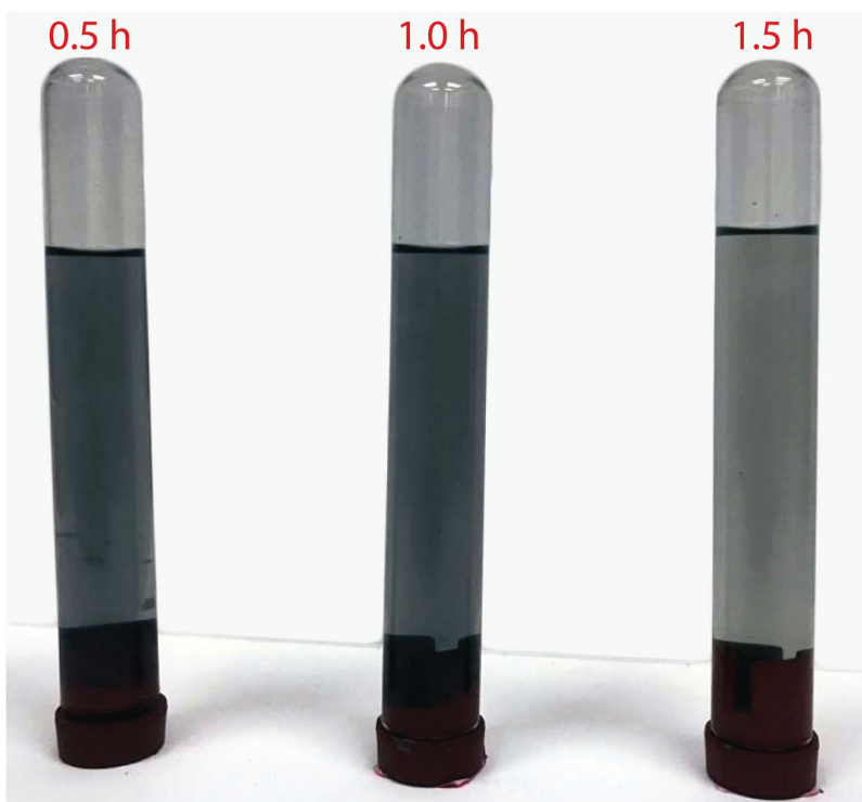
Figure S1. Optical images of rGO (black) suspensions. To obtain suspensions from rGO powder, the reduction of GO with CA was carried out considering three different times (0.5, 1.0, 1.5 h) with the procedure outlined in the main text. Then, 10 mg of rGO powder were added into 10 ml distilled water and sonicated for 30 min. The obtained suspensions were centrifugated for 30 min at 3000 rpm.
