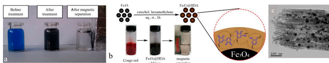
Figure 3. (a) Camera images demonstrate the various stages of water decolorization by the magnetic nanoparticles. Reproduced with permission [55]. Copyright 2016, Elsevier. (b) The schematic shows the synthesis procedure of the amino-coated \text{Fe}_3\text{O}_4 nanoparticles and their adsorption efficiency for the CR dye model. Reproduced with permission [56]. Copyright 2018, Elsevier. (c) TEM image implies embedment of Fe/Ni magnetic nanoparticles within the mesoporous carbon. Reproduced with permission [57]. Copyright 2015, Elsevier.
