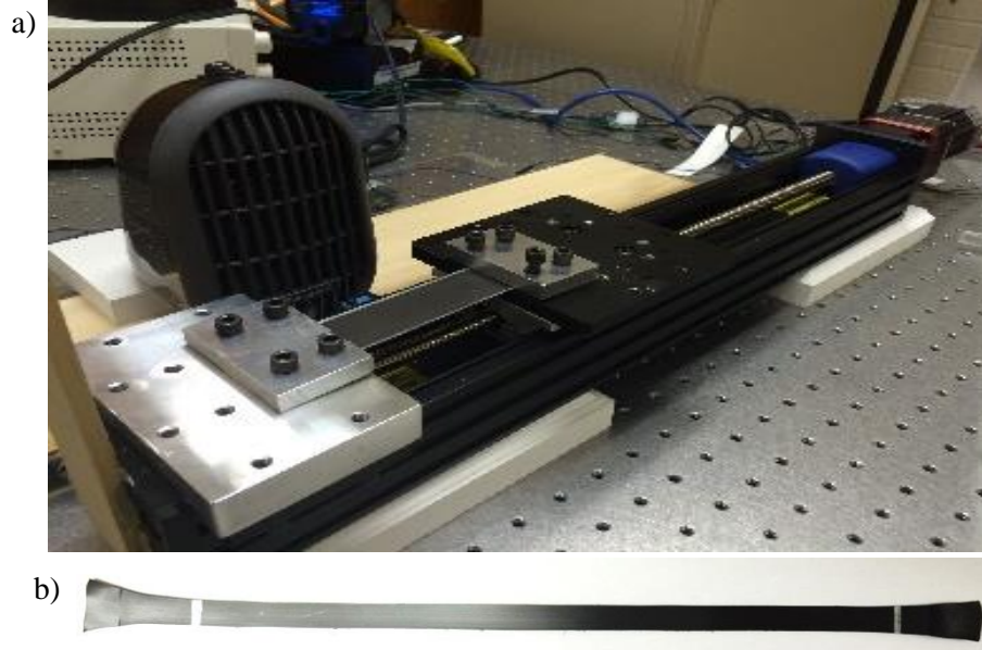
Figure S2: a) Experimental setup for stretching PE-GnP composites b) Stretched PE-GnP specimen.
