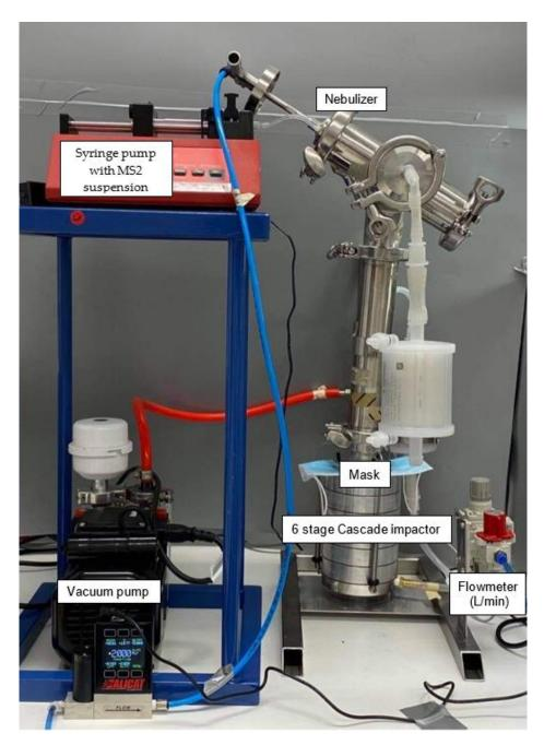
Figure 2. Mask testing rig, set up according to the ASTM F2101-14.
