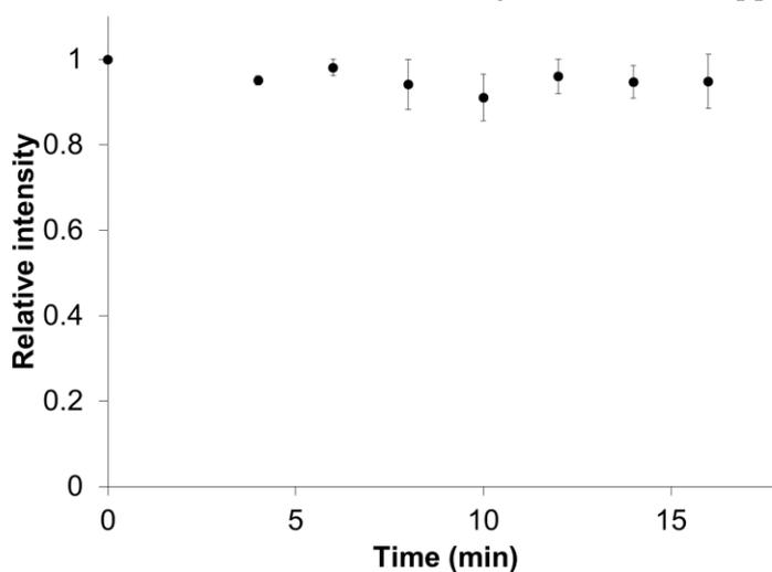
**Figure S2.** Time course of <sup>19</sup>F NMR signal intensity of <sup>19</sup>F-R8 after addition to HL60 cells. The intensity is the value relative to the <sup>19</sup>F NMR signal of the initial <sup>19</sup>F-R8 in PBS. Notice that the <sup>19</sup>F-R8 signal intensity is conserved all the time, meaning no degradation of <sup>19</sup>F-R8 by the presence of HL60 cells.
