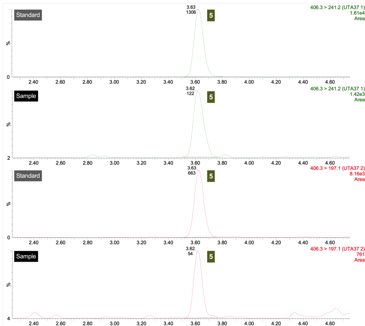
Figure S5. Exemplary mass spectrometry chromatograms for the metabolic conversion from the L -phenylalaninol derivative 3 to the L -phenylalanine derivative 5 . The detection and quantitation of 5 were performed using a H-Class UPLC-MS/MS system coupled to a XEVO TQ triple quadrupole mass spectrometer (Waters, NSW, AU). Analytical separation was carried out on a Waters Acquity UPLC BEH C18 column (2.1 × 100 mm, particle size 1.7 μm) at 30 °C. Mobile phases were 0.1% formic acid in purified water (A) and acetonitrile (B) with a flow rate of 0.3 mL min -1 . The final conditions included a gradient flow of mobile phase B: 40 % for 1 min, 40-90 % for 4 min, 90 % for 1 min, 90-40 % for 0.5 min, 40 % for 3 min (total run t = 9.5 min, including column post-conditioning). The mass spectrometer was operated in positive ionization mode, using electrospray ionization source (ESI). The tuning parameters of 5 were optimized by using a standard solution containing 8.11 ng mL -1 5 (20 nM in acetonitrile) with a flow rate of 20 μL min -1 to the mass spectrometer. Cell culture media collected (containing 40 μM 3 ) was precipitated by mixing 1:1 with acetonitrile, followed by 1:1000 dilution of the supernatant in acetonitrile to reach a theoretical concentration of 7.83 ng mL -1 3 (20 nM) for analysis. The standards and metabolized samples were detected by monitoring the precursor to product ion transition using Multiple Reaction Monitoring (MRM) scan mode with 78 ms dwell time for each transition. The selected transitions were m/z 406.3 > 197.1 and 406.3 > 241.2 for 5 . The source temperature was 130 °C, desolvation temperature was 450 °C, desolvation nitrogen gas flow was 950 L h -1 and cone gas flow was 50 L h -1 . The capillary voltage was set at 2.85 kV, while the cone voltage values for 5 were optimized at 27 V. The multiplier was set at 528 V and argon was used as collision gas. The optimized collision energies were 24 eV (392.2 > 152.1) and 16 eV (392.2 > 197.1), respectively. All data were required using MassLynx software (version 4.0, Waters, NSW, AU).
