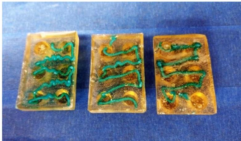
**Figure S3.** Soft dosage forms with paracetamol inside (blue line) fabricated via one-step e-3DP with printing speed 55.0mm/min.
