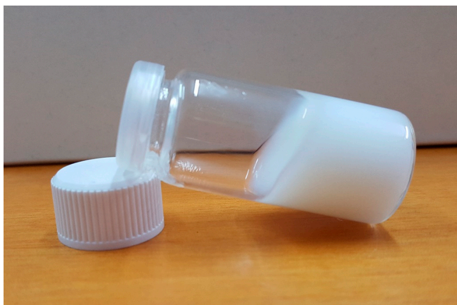
Figure S3. Appearance of the viscous 20% w/w Soluplus dispersion in PBS pH 7.4 at 37 °C.
