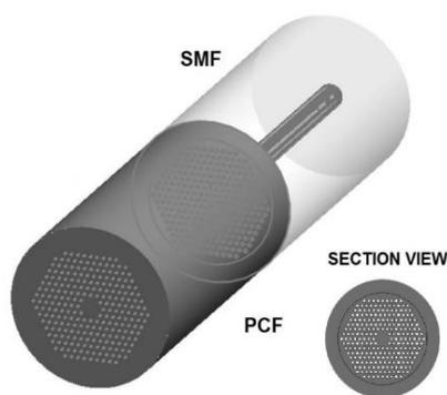
**Figure 2.** Refractometric fiber Fabry-Perot tip based on an endlessly singlemode PCF [25].
