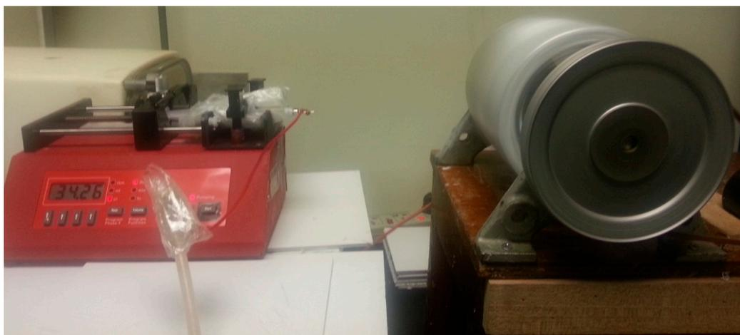
**Figure S1.** Electrospinning on the rotating drum in our lab (homemade).
