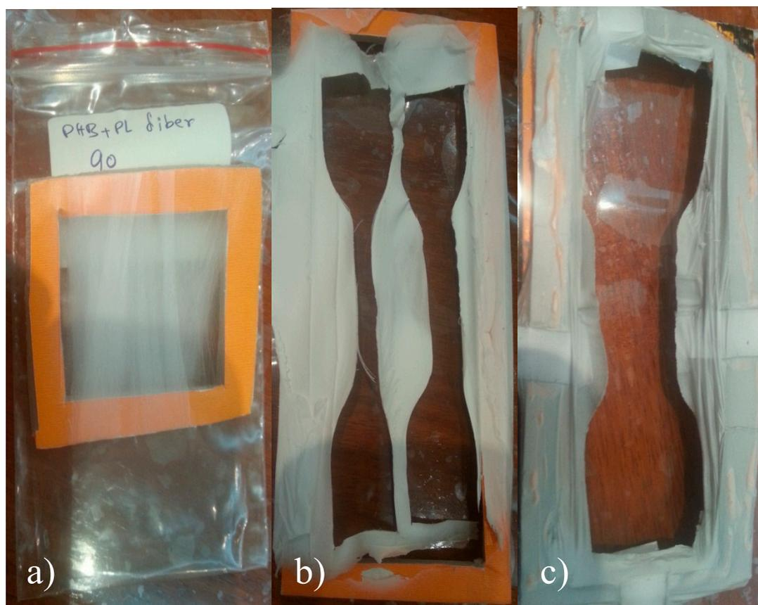
**Figure S3.** Fiber rolling after electrospinning processes on the frame and the method to collect by the frame for the dumb bell shape.
