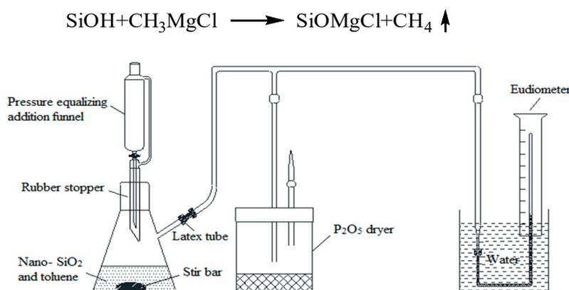
Figure S1. Flow-process diagram of CH<sub>3</sub>MgCl titration.
