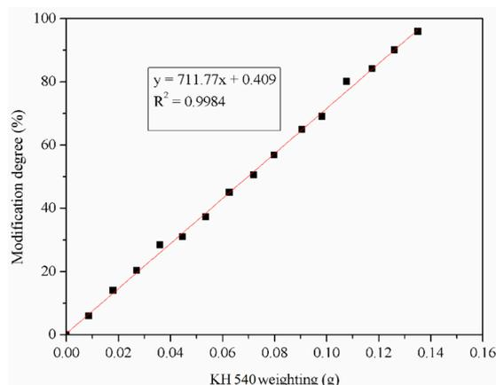
**Figure S2.** Effect of KH540 dosage on surface modification degree of nano-SiO<sub>2</sub>.
