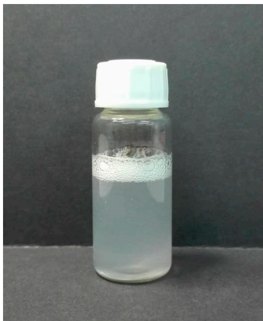
Figure S3. The photo of aqueous solution of the synthesized diblock copolymer PNIPAM- b -PS (a solution of sample PNPS3). As the molecule of PNPS3 is amphiphilic characteristic foam appears as a result of surface tension decreasing.
