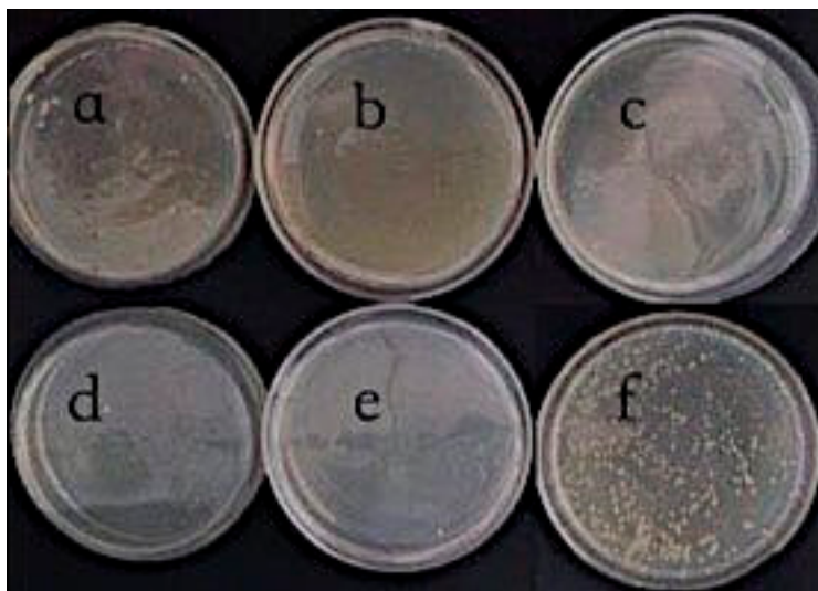
Figure 4. Photographs of antibacterial activity of CS/Gr modified bamboo fiber fabrics (CGBFs). (a) C1G1; (b) C1G2; (c) C1G3; (d) C1G4; (e) C1G5; and (f) control sample.
