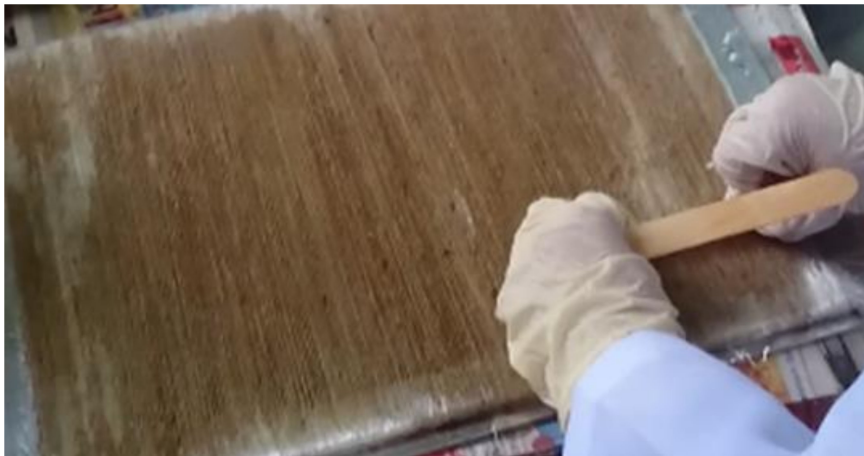
Figure 3. The example of a unidirectional kenaf fiber reinforced polymer (KFRP) composite sample after the curing process.
