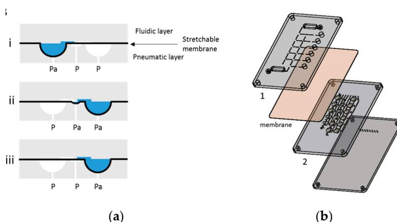
**Figure 1.** Hybrid cartridge made from 2 plastic cards and a stretchable membrane. (a) Schematic cross sectional view of fluidic actuation; (b) Perspective view of cartridge technology.
