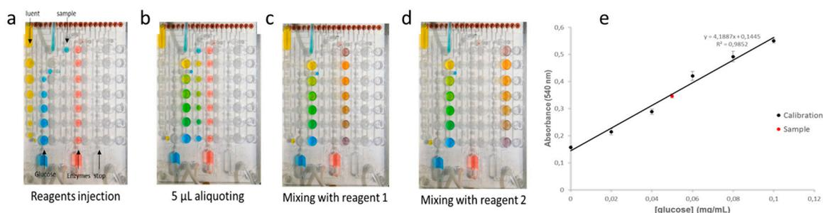
**Figure 3.** Validation of glucose assay with on chip calibration curve: Protocol steps (a–d). Plots of absorbance intensities at 540 nm depending on the dilution factors (e).
