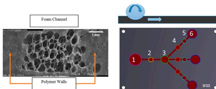
**Figure 2.** SEM image of a foam channel section. The liquid can flow through the porous matrix soaked in polymer (a). Top view of a fluidic pathway designed for a blood typing test. A rolling actuation induces the transport of biological samples through successive reservoirs (1: buffer; 2: blood; 3: mixing; 4: specific typing antibodies; 5: hollow chambers for visualization; 6: wastes).
