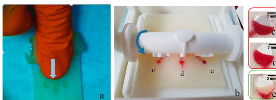
**Figure 4.** Blood typing test in fully flexible foam-based microdevice which can be manually wrapped for the generation of a Poiseuille flow (a); similar effect is obtained with a roller (b); Specific typing antibodies embedded in the device allow visualization of the blood type—negative (c,d); positive (e)—in dedicated hollow chambers.
