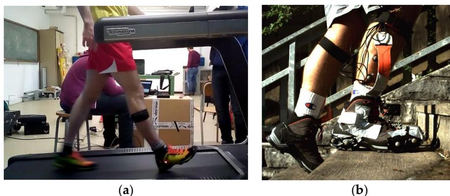
**Figure 3.** Data collection sessions: (a) example of data collection of one subject wearing TR shoes, walking at 5 km/h on a treadmill with an inclination of 5%; (b) example of data collection of one subject wearing CH shoes climbing a flight of stairs outdoor. Both IMU and video based acquisition systems were used together.
