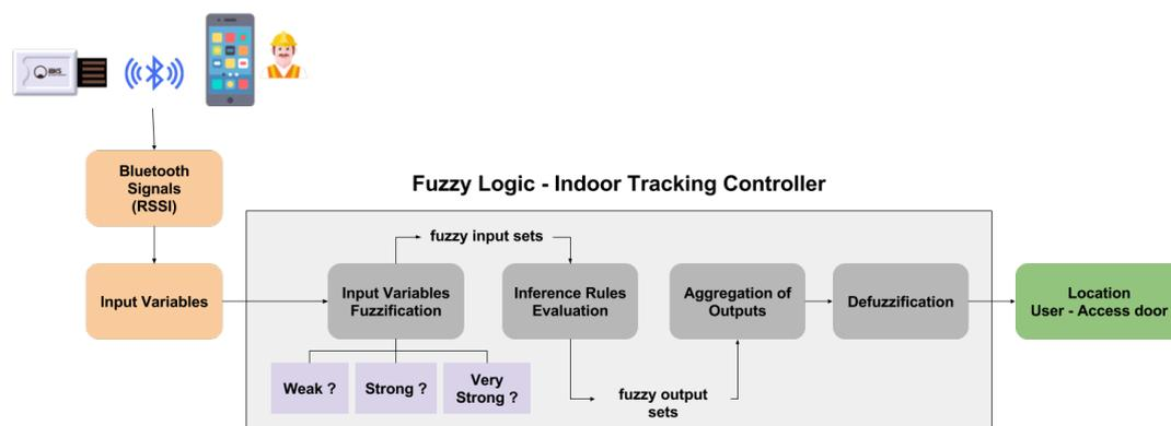
Figure 2. Fuzzy Indoor Tracking Controller
