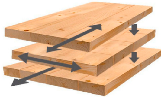
Figure 1. Cross-laminated timber configuration. ( https://www.sfhac.org/mass-timber-wood/ ).
