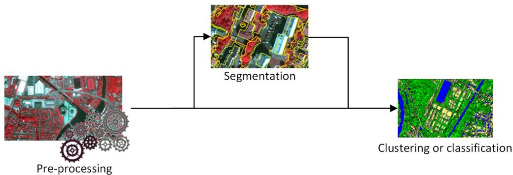
**Figure 2.** The 3 steps of satellite image processing.
