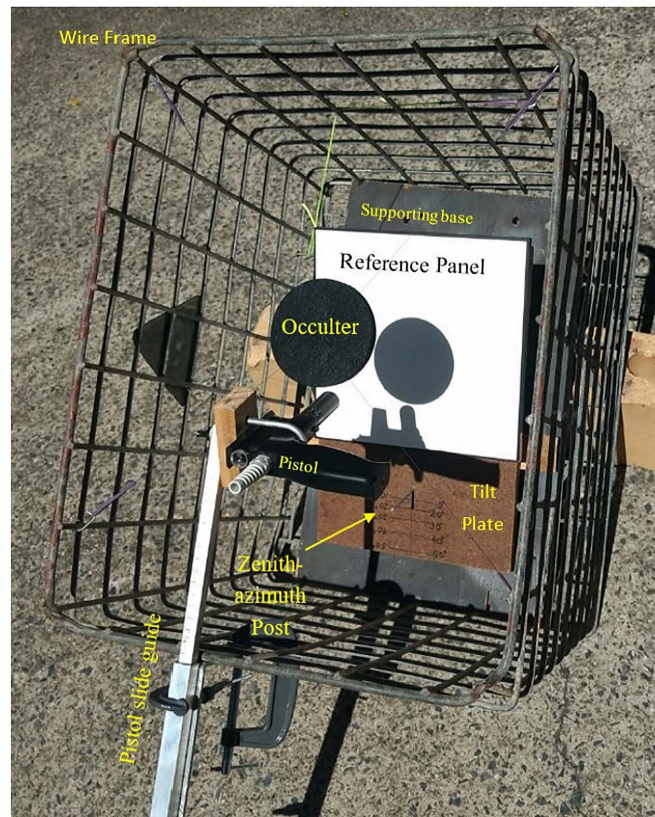
Figure 5. Field setup showing wire frame, black supporting base, brown tilt plate, reference panel, occulter, zenith/azimuth post set at 20^\circ zenith, spectrometer pistol, and pistol guide slider to ensure accurate spacing of signature capture.
