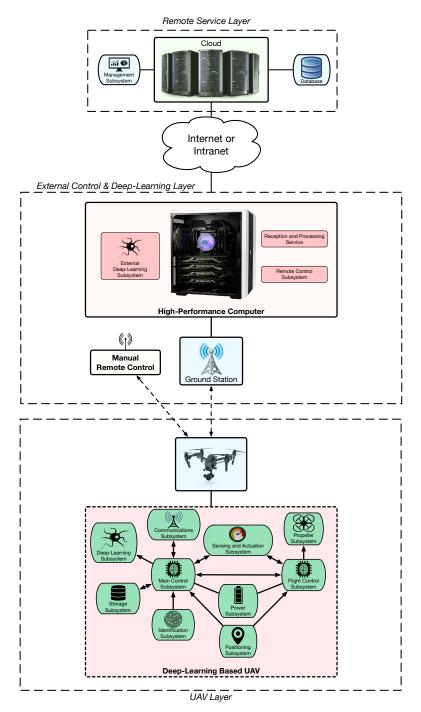
Figure 1. Typical cloud-based deep learning UAV-based communications architecture.
