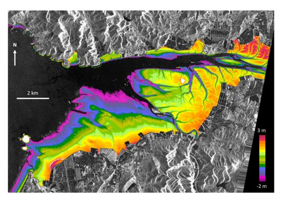
**Figure 5.** TanDEM-X (TDX) interferometric synthetic aperture radar (InSAR) digital elevation model (DEM) for the Gomso Bay test site. The estimated DEM (color) for the tidal flat is overlaid on the TDX amplitude image (grey), scaled from -2 to 3 m. Upper left:  $35.710139^{\circ}N/126.46995^{\circ}E$ . Bottom right:  $35.610046^{\circ}N/126.64958^{\circ}E$ . The extent of the DEM image is 11.1 km (N-S)  $\times 16.3 \text{ km}$  (E-W) and the spatial resolution of the DEM is 5 m (from [19]).
