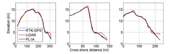
**Figure 2.** Three beach profiles showing the comparison between RTK-GPS, Pleiades (PL1A) and LiDAR, showing the erosion of the berm that occurred between the LiDAR survey and RTK-GPS and Pleiades (from [17]).
