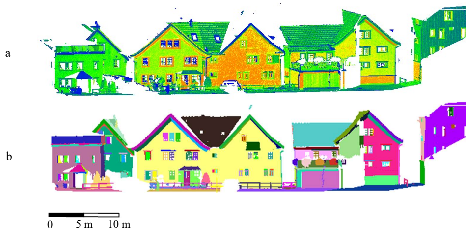
Figure 8. Terrestrial light detection and ranging (LiDAR) data. (a) Point cloud published by Zurich Federal Institute of Technology (ETH) Zurich, and (b) ground truth data obtained by manual segmentation.
