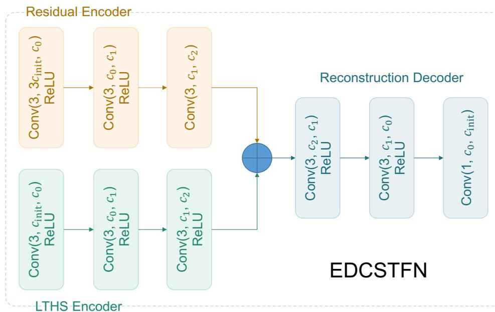
**Figure 4.** The detailed design of EDCSTFN model for MODIS-Landsat fusion (the three parameters of a convolution are kernel size, input and output channels; the kernel size is empirically set to 3 except for the last layer. The  $\oplus$  denotes element-wise addition of multi-dimensional arrays).
