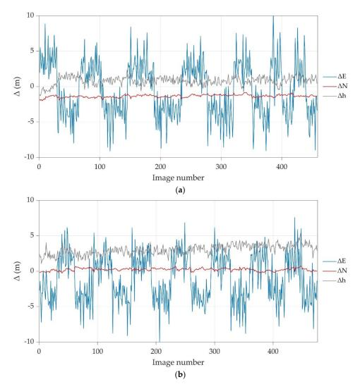
**Figure 3.** Differences ( $\Delta$ ) between the single-frequency and dual-frequency exposure (camera) position estimates for: (**a**) the first flight, and (**b**) the second flight ( $\Delta$ E—easting,  $\Delta$ N—northing,  $\Delta$ h—altitude). Differences ( $\Delta$ ) are expressed in HTRS96/TM (ESPG: 3765).
