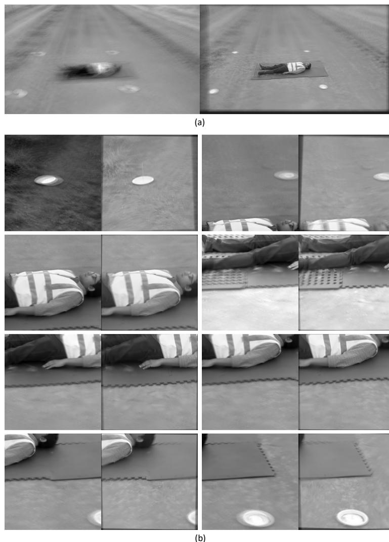
**Figure A1.** Some selected mean images after the video stabilization of video A1. (a) The raw input mean (left) and corrected sequence mean (right) of video A1. The corrected sequence mean is calculated after the first level of stabilization. (b) Mean images after the second level of stabilization. Each pair of images represents the raw input mean (left) and corrected sequence mean (right) of a randomly selected tile video of A1.
