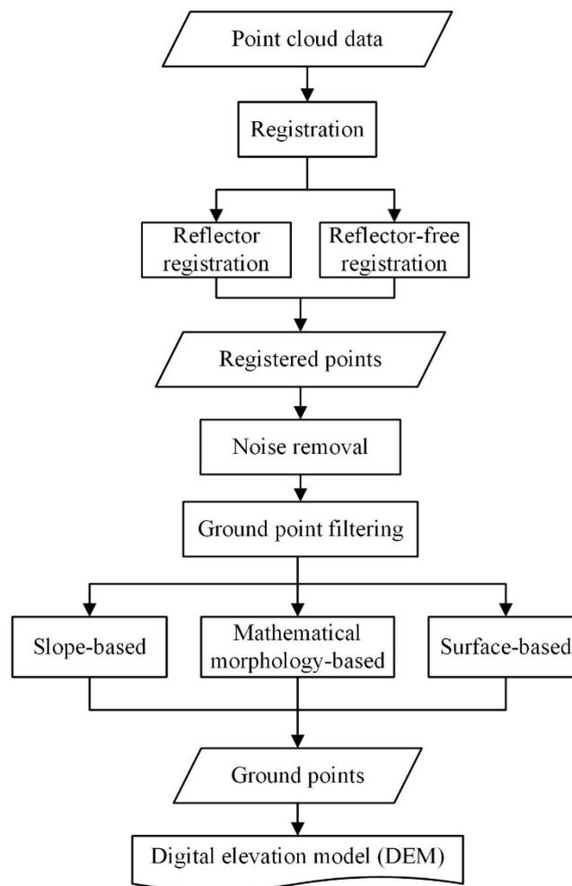
Figure 5. Preprocessing of the point cloud data.
