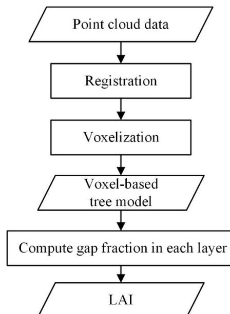
**Figure 8.** Estimation of LAI from point cloud data with the 3D method.
