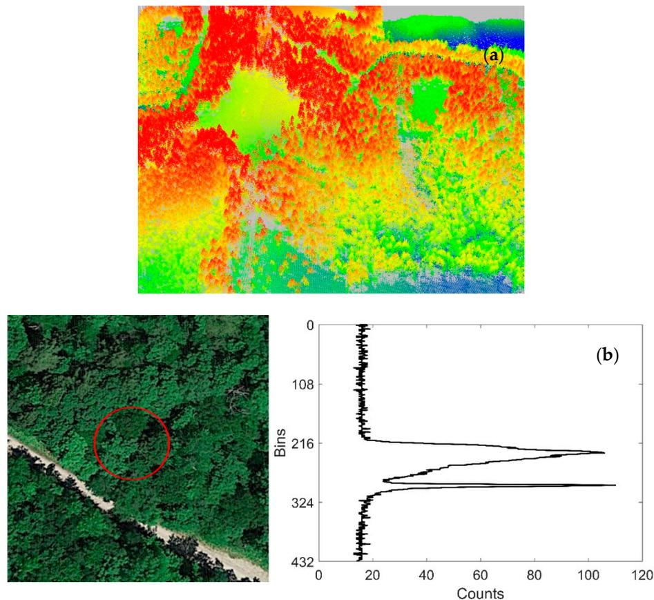
**Figure 3.** Airborne laser scanning (ALS) data examples. (a) Airborne point cloud data colored by height (4.3 points/m<sup>2</sup>); (b) airborne large-footprint full-waveform data—Land, Vegetation, and Ice Sensor (LVIS)—~20 m in diameter (44°2′59″ N, 71°17′18″ W), 2009 [46]. The image in the left panel is from Google Earth®, and the right panel is a waveform return where the upper and lower peaks come from the forest canopy and the ground surface, respectively.
