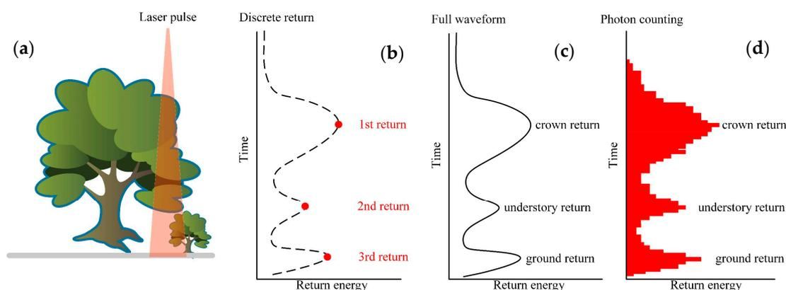
**Figure 1.** Conceptual diagram of different light detection and ranging (LiDAR) systems (signals returned from trees and the ground). (a) Intersection of the laser illumination area with the tree crown and signals received with the (b) discrete return, (c) full waveform, and (d) photon-counting LiDAR systems.
